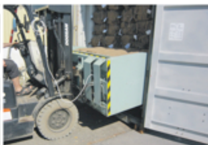
Loading container with Easy Container Stacker
